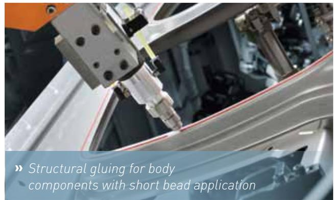
» *Structural gluing for body components with short bead application*
